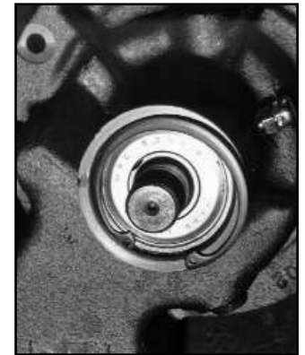
VHO-206 retaining water pump shaft in housing.
