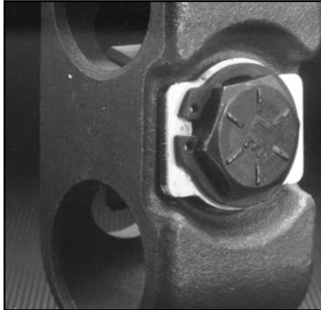
SHR ring retains this plate on tank tread linkage.
