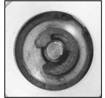
HOI with inverted lug provides better clearance for E ring (center) on this automatic transmission spool valve.
