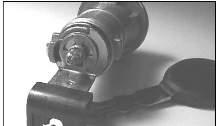
BE retaining ring on a car ignition starter assembly.
