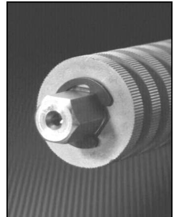
E ring retains the cutters on a shaft used on a paper shredder.
