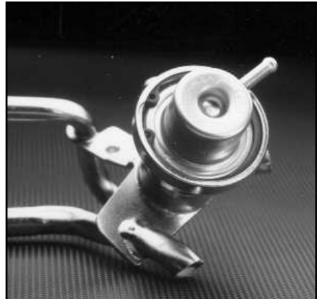
HO internal ring retains the valve of this fuel rail assembly.
