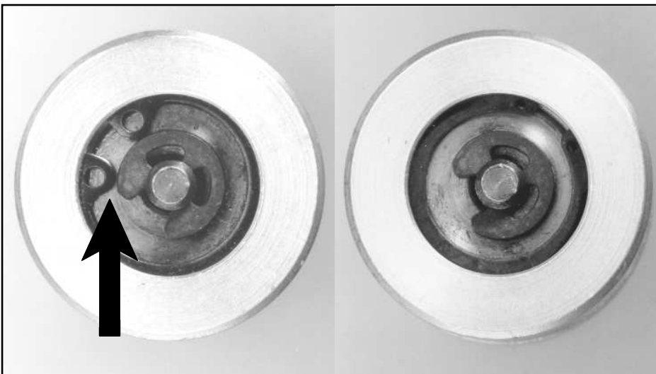
When clearance seemed to be a problem between this E ring (left center) and the lugs of the HO ring, the manufacturer switched to an HOI version with inverted lugs (right) for this automotive transmission spool valve.
