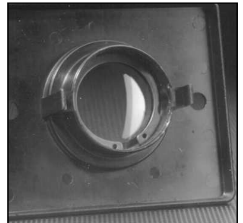
HOI retaining ring differs from the standard HO in that the lugs are inverted. The ring retains the assembly while allowing another component to pass without interference from the lugs.
