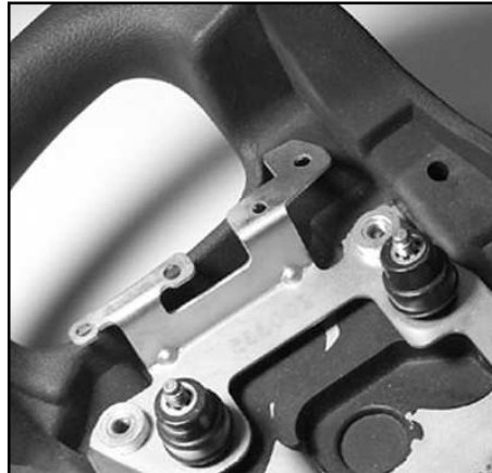
Two external, self-locking TX rings on an automotive steering wheel assembly.
