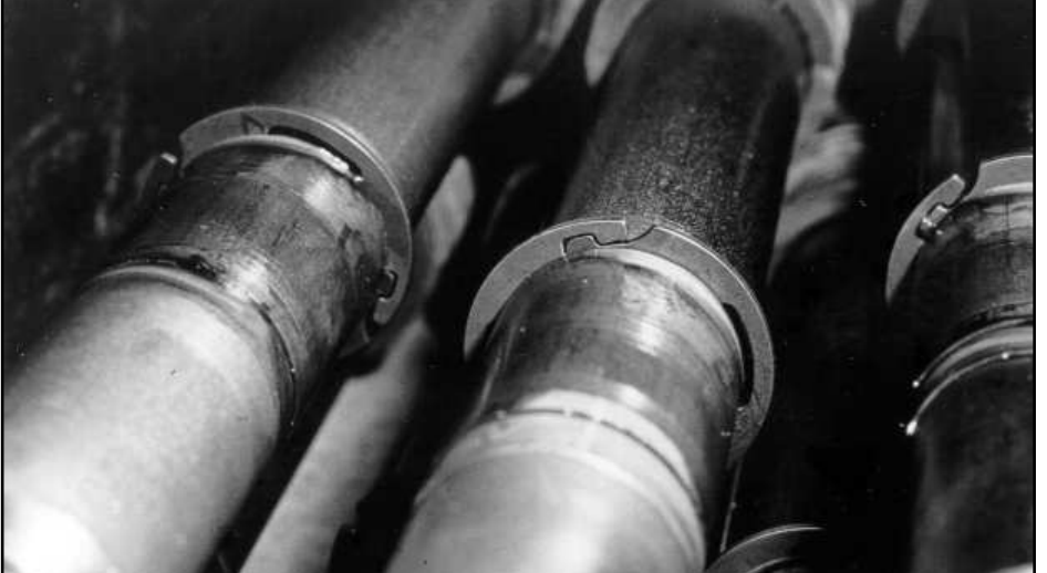
Two part LC ring is dynamically balanced once installed, making it very effective in retaining this escalator assembly during high rotational speeds.
