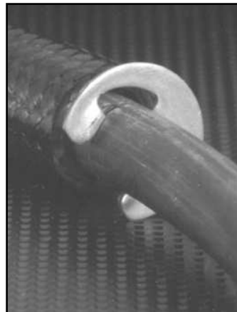
An RE ring cuts into the hard plastic cable coating and provides a shoulder to hold a protective sleeve in place on a transmission.
