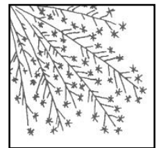
SAE 1060-1090 Long straight streamer with star-shaped burst.
