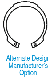
Measuring Free Diameter (Df) HOI Series Df = D1 + 2(S \text{ max})
