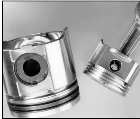
A standard HO retaining ring (left) is easier to assemble/disassemble than wire formed version (right.)
