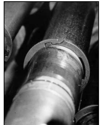
Two part LC ring is dynamically balanced once installed, making it very effective in retaining this escalator assembly during high rotational speeds.
